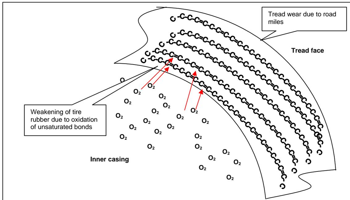
the casing, and closer towards the outside of the tire, including the tread face. At some stage the two surfaces meet. The outer tread wear face comes into contact with the degraded rubber layer. At this point, the durometer hardness of the rubber changes, and typically tread wear accelerates. The remainder of the tread wears at a much faster rate than the new tread did. This phenomenon is shown in the following chart.
