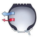
Because air can migrate through sidewalls, truck tires can lose up to 2 psi per month, even when valves and beads seal properly and there are no punctures.
